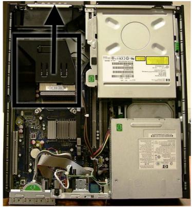
To install the baffle, reverse the removal procedure.
